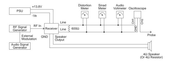
Figure 3.2 Test Equipment Set-up
